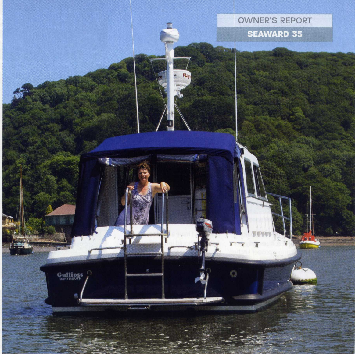
A low freeboard and wide decks make getting about onboard safe and easy. A ladder aids those who fancy a swim
