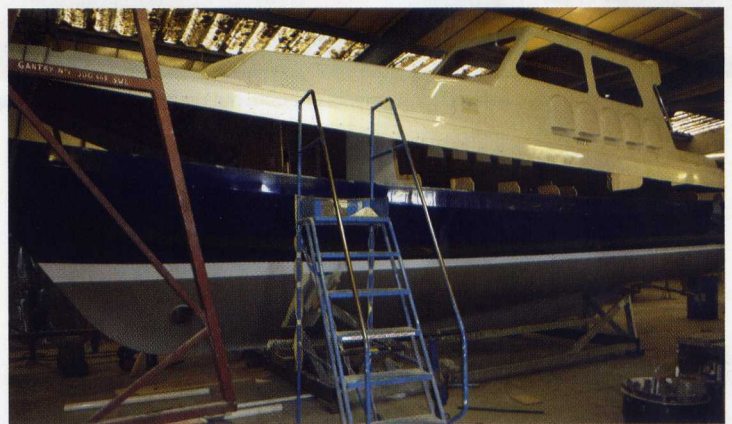
Gullfoss takes shape as the superstructure is lowered on to the hull
